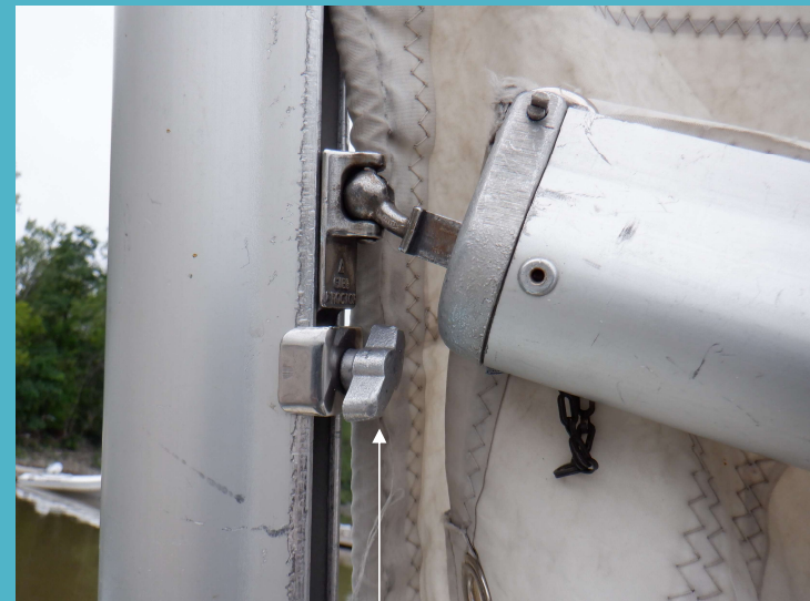
Butterfly nut: Adjust height of the boom
