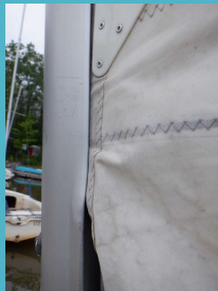
Bolt rope slide into groove of the mast
